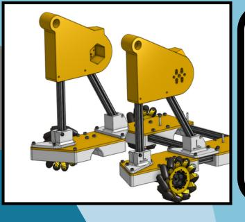
The final pieces of the bot are the pivot structures shown in yellow on the left. These structures are held up by the REV shafts and provide support to both the catapult motors and the final wheel of the intake chain. These were the hardest elements to print as they had support filament on the inside of the cutout for the REV shaft, though this bot was fairly easy to print as a rule.
