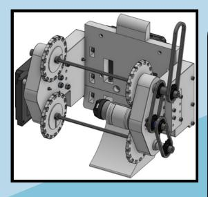
All of these individual systems come together to create an intake which can funnel the 5" diameter balls from ground level to 18" in the air in a matter of moments. Powered by only one motor, this intake is cheap and easy to fix/improve. Not only that, but limited total parts equals limited parts to possibly fail. From here, the artifacts fall into the hopper ready to be launched by the catapult. We hope to innovate upon this design over the next month.
