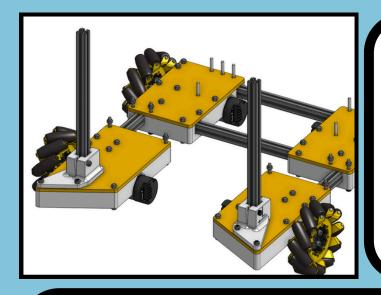
Our chassis was unique in its design as it did not rely on a full metal structure, but a mix of 3D printed clamshells and the REV 15mm shafts they held. Because of the relatively low weight of the full bot ≈20lbs this system worked well. The motors were mounted with a mix of 10mm bolts with 8mm washers and 1/4" zip ties which wrenched them to the frame.
