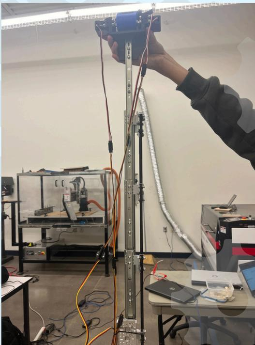
The height of the arm when fully extended is approximately 260 mm, but it is still not sufficient to reach the tallest basket. To address this, we plan to extend the arm slightly in order to ensure it can reach the highest basket.
