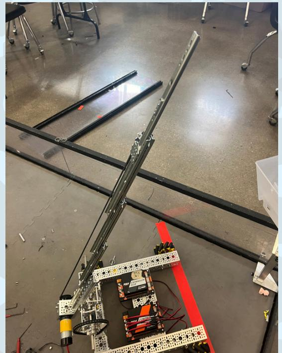
The hook is currently too large, which causes it to interfere with the claw, preventing the arm from fully retracting and staying out of the way. This also affects the functionality of the hooks, making them unable to operate correctly. Additionally, the wires need proper connections to ensure they function as intended.
