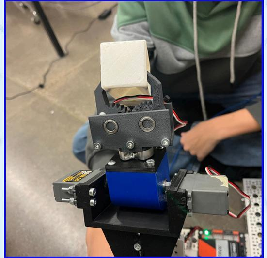
A rotating arm that picks up blocks using a bevel gear system relies on a motor to drive the motion through gears arranged at an angle. The bevel gears transfer rotational motion from the motor's shaft to the arm, which is mounted on another shaft. In this setup, the bevel gear system physically transfers the rotational motion from the motor to the arm. While the bevel gears affect the speed and torque of the arm, they don't require changes to the code, as the system operates mechanically.
